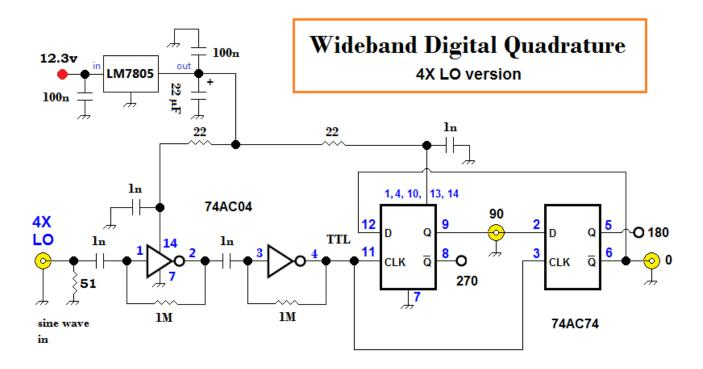
If signal generator has square wave output with 50/50 duty cycle and TTL -- just connect to flip-flop
