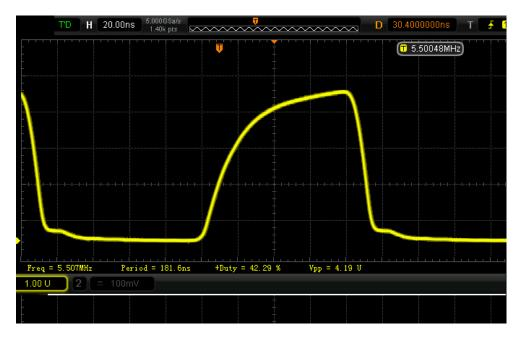
Above – The output from the BJT sine to square wave converter.
