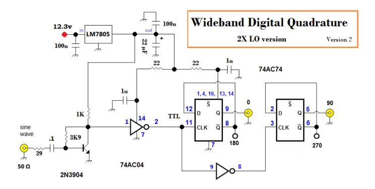
Above --- Version 2 of the 2X LO with a BJT sine to square wave converter and a single inverter to square it up.
