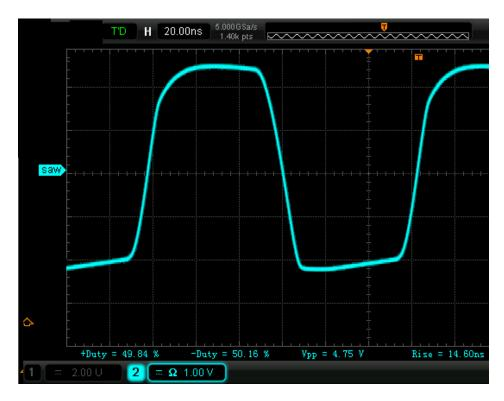
Above – The duty cycle corrected towards 50%. Then, I connected up **1** inverter from a 74AC04 used in the quadrature stage to square it up.
