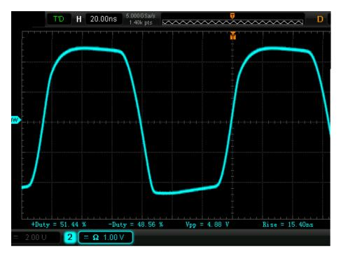
Above - A 51.44 – 48.56 duty cycle from the differential circuit with 1 setting of the 5K trim pot
