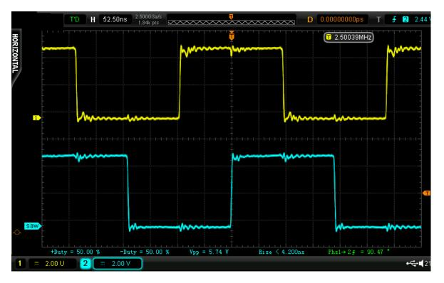
Above --- The quadrature output where LO = 5 MHz. I got a little closer to my goal of 0 degrees phase error. I was able to slightly tweak for lower phase error with the pot on the differential
