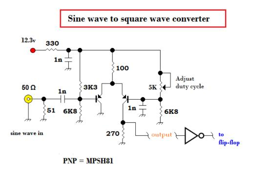
Above – Differential circuit. By placing a trimmer pot on the BJT with its base AC grounded, I found you can vary the duty cycle a little.
