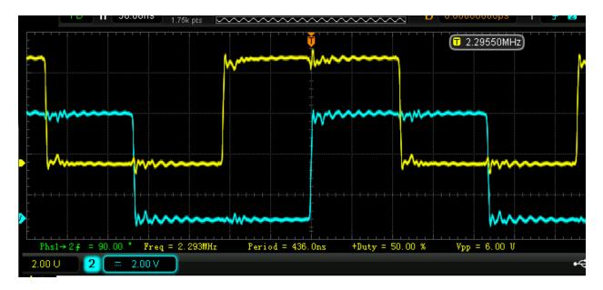
Above – At frequencies ~2- 5 MHz, I was able to obtain zero degrees phase error by tweaking the sine wave signal source. Moving above 5 MHz, phase error slowly crept in.
