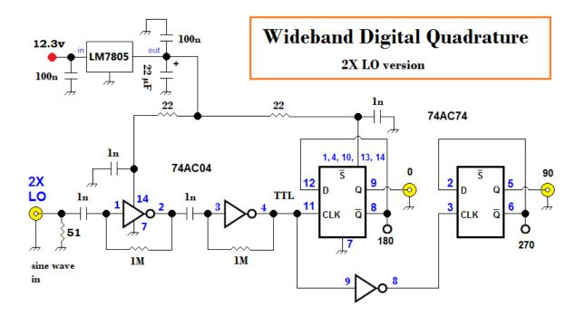
If signal generator has square wave output with 50/50 duty cycle and TTL -- just connect to flip-flop
