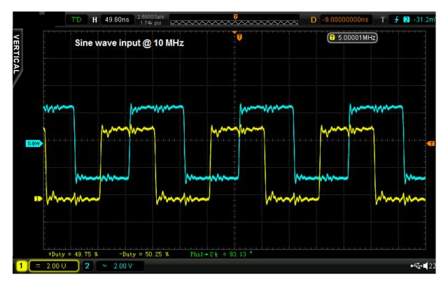
Above -- the quadrature output with the sine wave oscillator set to 10 MHz. I measured a 3.13 degree phase error. That would trash opposite sideband suppression on 30 meters. I then investigated varying the duty cycle on the sine wave to square wave converter. Although digital circuits with feedback that allow a varied duty cycle may be found in the literature; to alter the duty cycle, I went to a simple differential circuit I learned about from Charles Wenzel.
