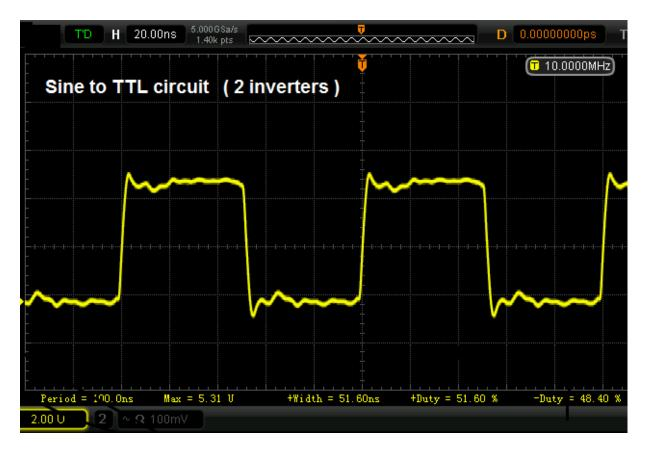
Above – The output of the 2 inverters when driven with a sine wave with the D-FF disconnected. Not quite a 50/50 duty cycle.
