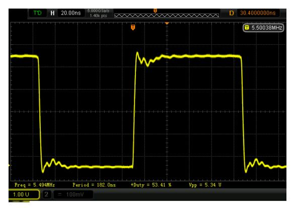
The output from the inverter that follows the BJT. By tweaking the sinewave signal source drive pot ( between 8 - 10 dBm ), I was able to affect the duty cycle of the square wave output
