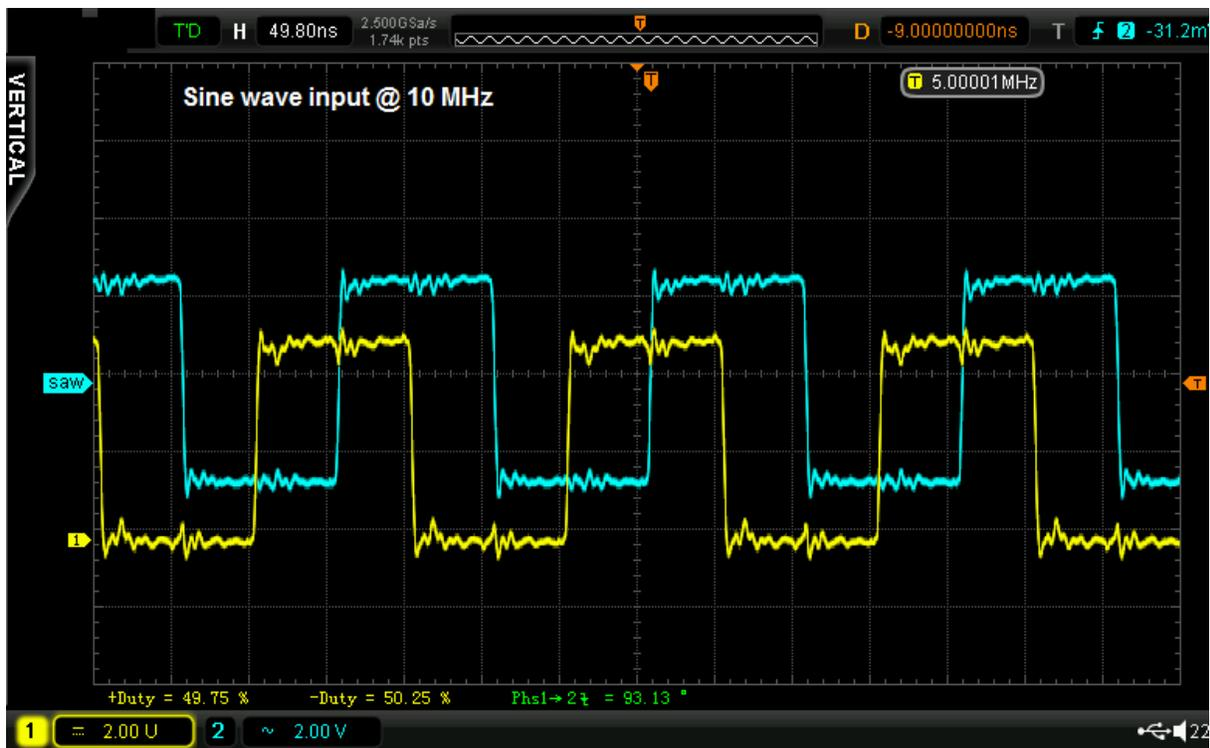
Above -- the quadrature output with the sine wave oscillator set to 10 MHz. I measured a 3.13 degree phase error. That would trash opposite sideband suppression on 30 meters. I then investigated varying the duty cycle on the sine wave to square wave converter. Although digital circuits with feedback that allow a varied duty cycle may be found in the literature; to alter the duty cycle, I went to a simple differential circuit I learned about from Charles Wenzel.
